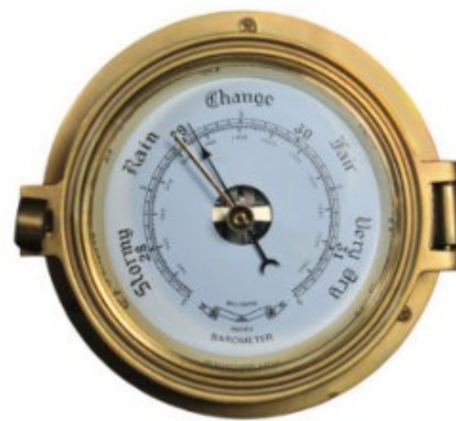
A barometer measures changes in atmospheric pressure and helps to predict whether it will be wet or dry.
